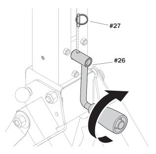
**3.** Remove the crank handle assembly (26).
